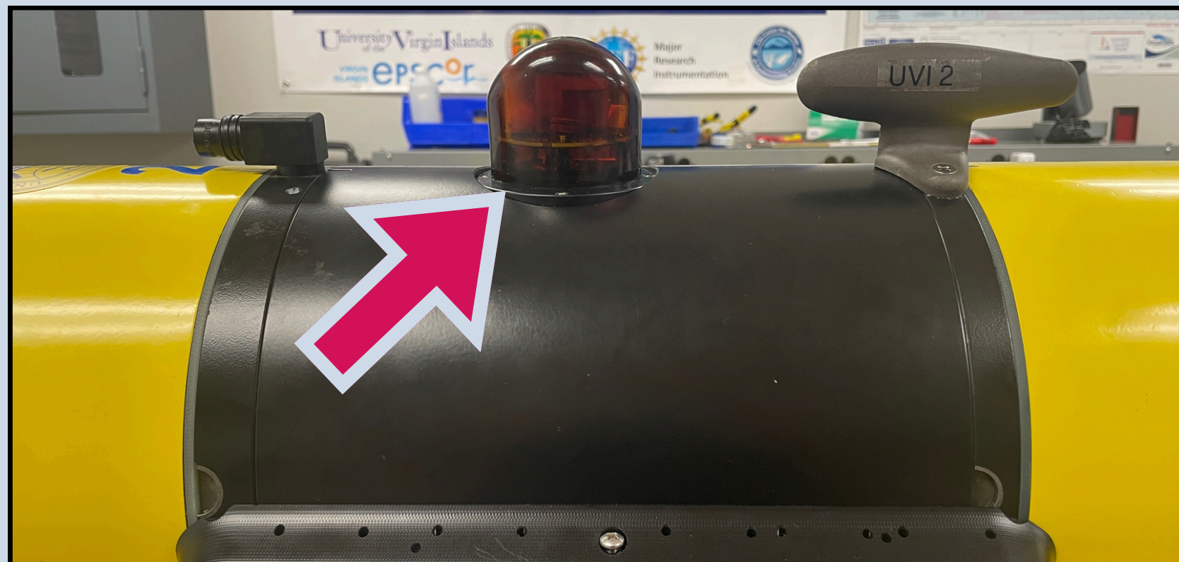
Figure 4. The external portion of the DMON2 system, attached to the science bay of a TWR G3 Slocum glider. This epoxy dome encapsulates three hydrophones: low, medium, and high frequency recorders.
